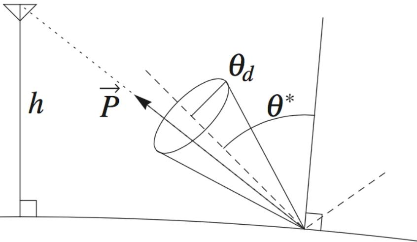
Fig. 1. Geometry of cosmic ray detection by a high altitude antenna.
