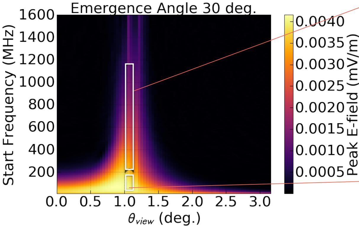
Narrowly peaked ( $\sim 1^\circ$ ) Cherenkov cone at high frequencies. Broader ( $\sim 2.5^\circ$ ) degrees at lower frequencies
