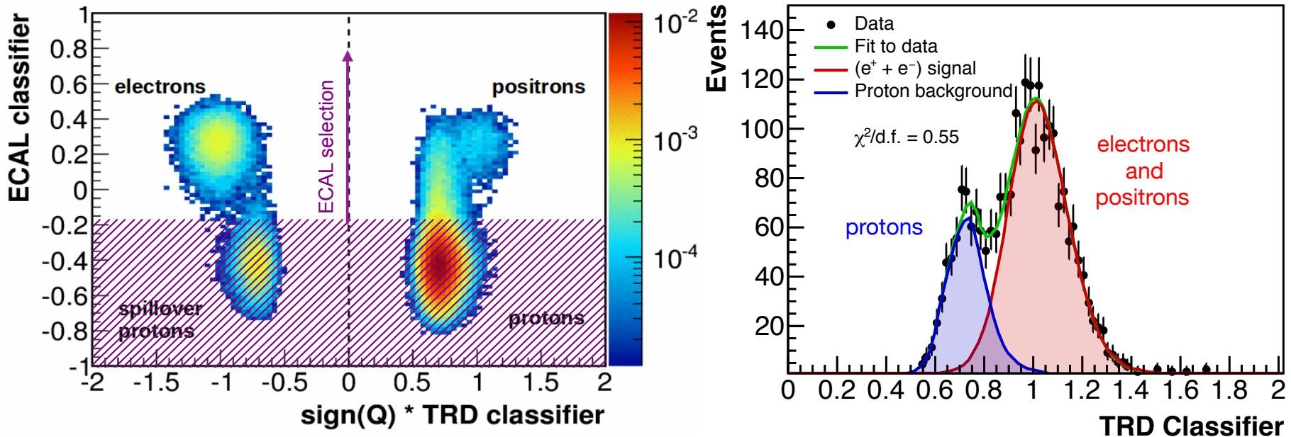
Measurement is performed for the cut on the ECAL classifier that minimizes the overall statistical + systematic uncertainty
