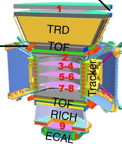
Thanks to the different energy deposits of light and heavy particles, the TRD is capable to achieve an e/p separation up to  $10^4$
