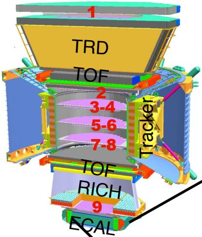
Exploring the shower topological differences between hadronic and electromagnetic particles, is possible to obtain an e/p separation up to  $10^5$
