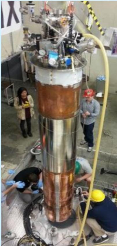
High Q cavity, magnet, dilution refrigerator (new)
