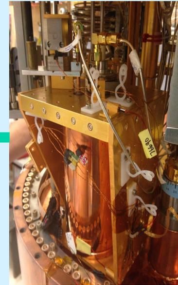
Small cavity prototype “sidecar” taking data 5-7 GHz **now**. First thesis on the 5 GHz data completed. JPA’s.
