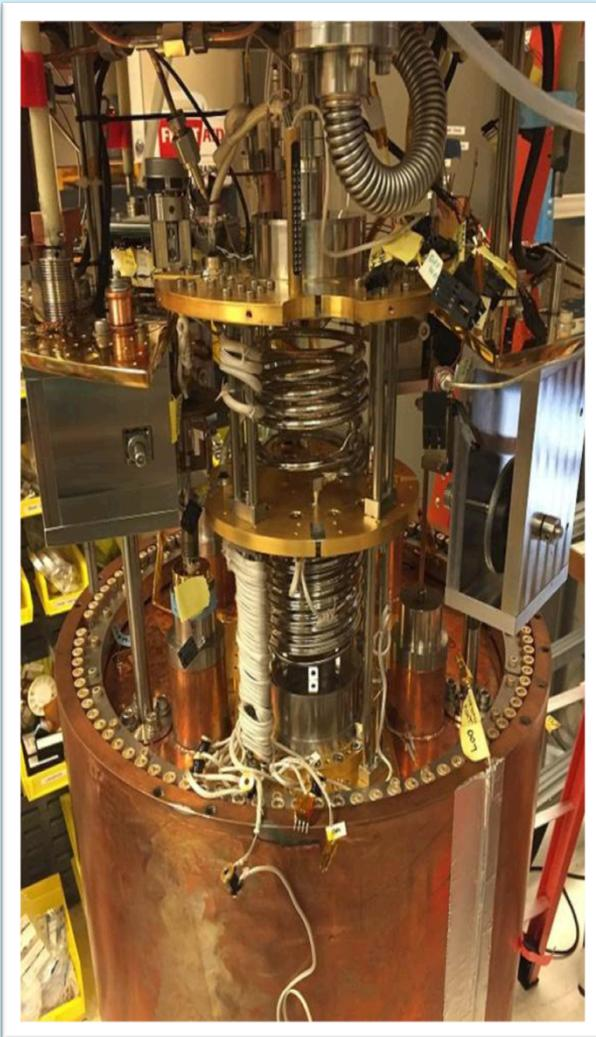
Dilution Refrigerator installed above ADMX Cavity
