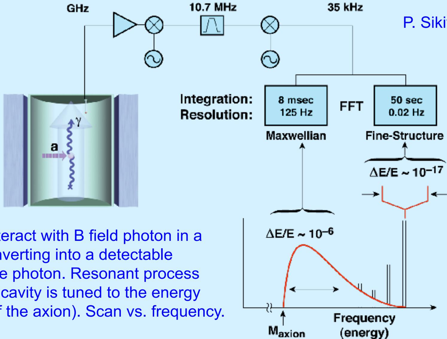
Axions interact with B field photon in a cavity converting into a detectable microwave photon. Resonant process when the cavity is tuned to the energy (i.e. KE of the axion). Scan vs. frequency.
