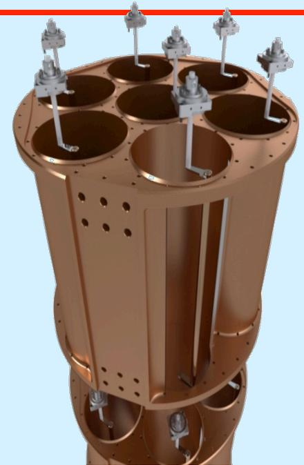
Multicavity systems for 2-4 GHz designs being finalized.
