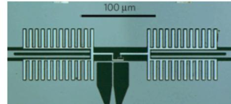
Superconducting qubit in field-free bucking coil region acts as an amplitude  $\rightarrow$  frequency transducer for QND measurements.
