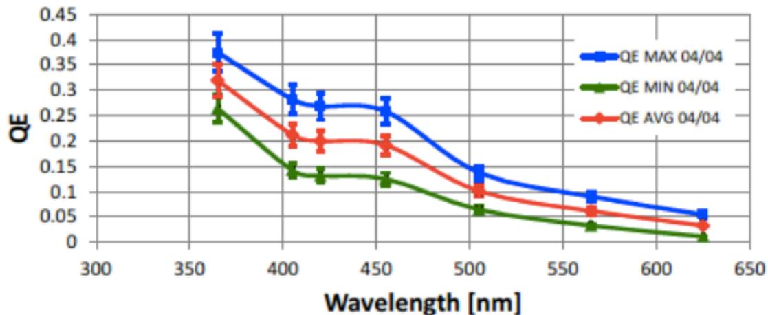
The average QE at 375 nm remains at 30%, with a maximum 35% and minimum of 22%
