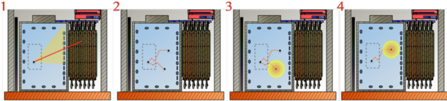
1. CC interaction in the fiducial volume produces a muon, reconstructed in the water volume and MRD.
