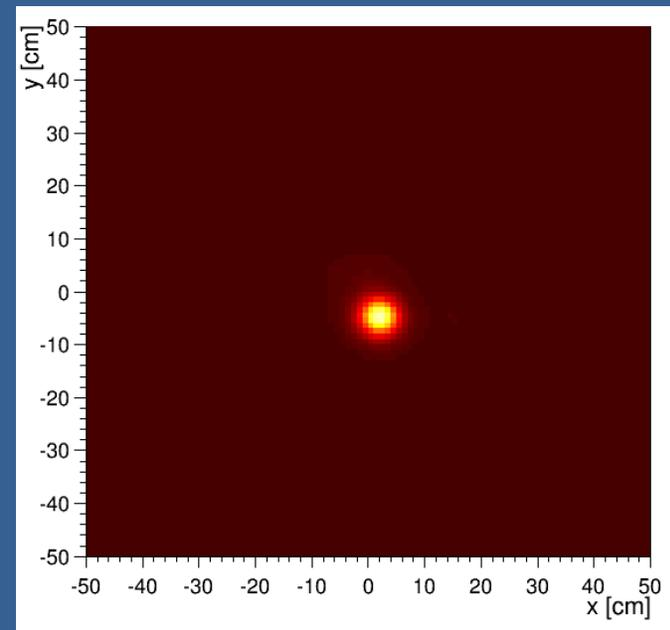
Calibration image of a 662 keV  $^{137}\text{Cs}$  source  $\sim 56$  cm above the instrument.
