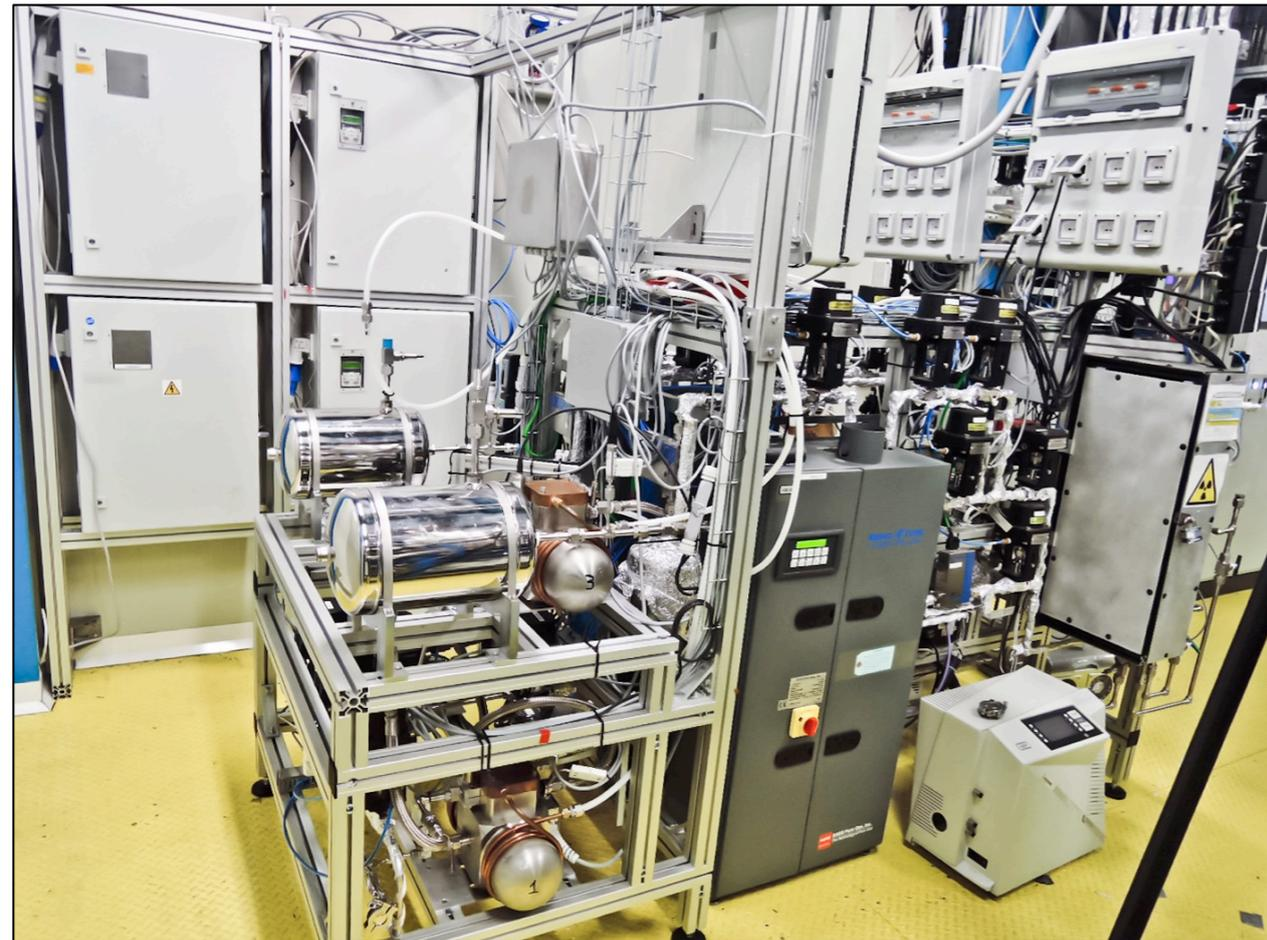
**Goal:** remove electronegative impurities below 1 ppb (O<sub>2</sub> equivalent) in the Xe gas fill and from outgassing of detector's components with continuous circulation of Xe gas at high speed through hot getters
