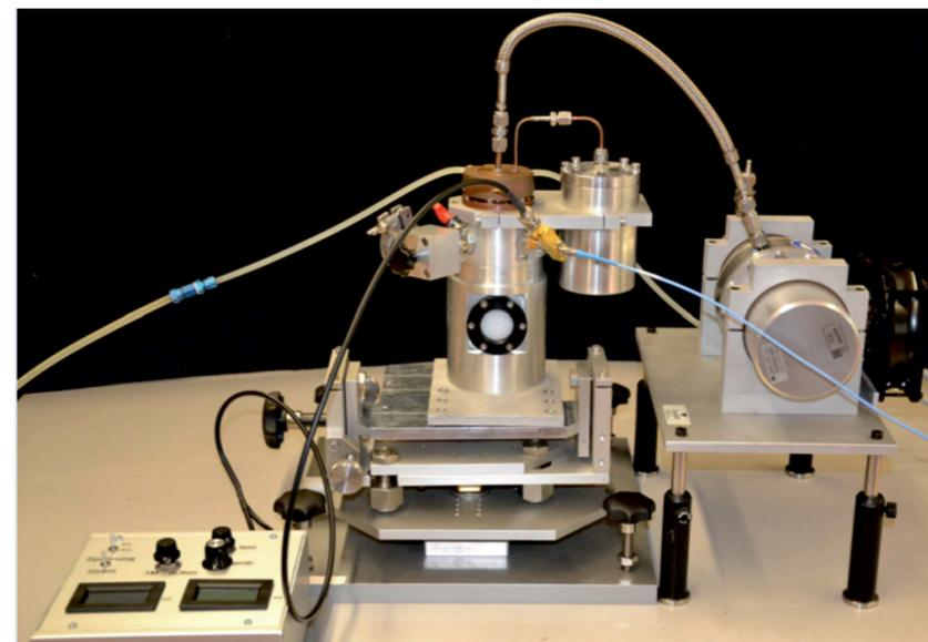
*THz detector developed at KIT (LN2)*
