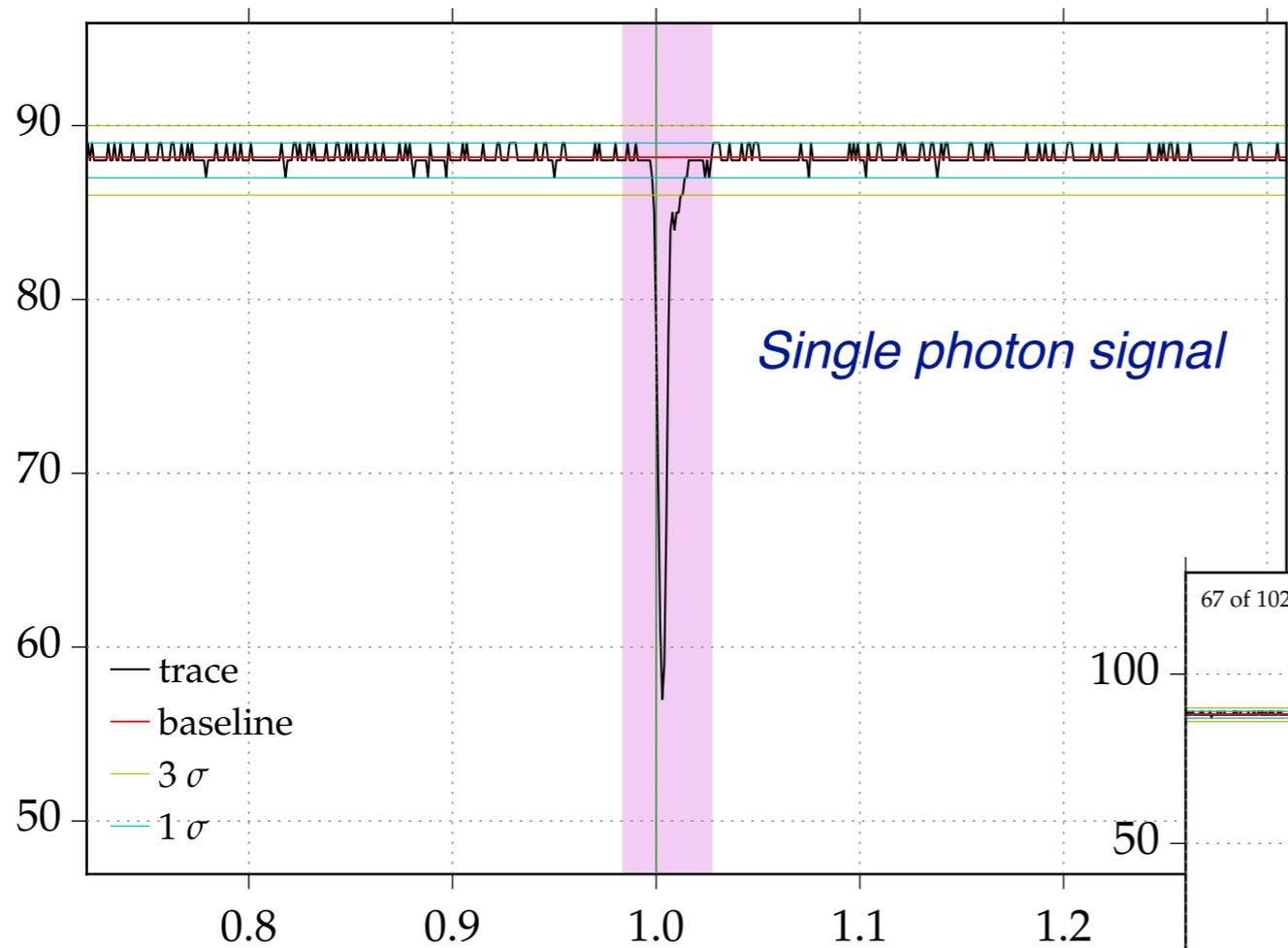
Trace of 2000 bins of 0.8 ns size (800  $\mu$ s before and after trigger)
