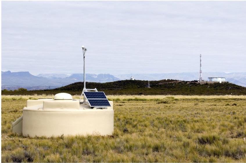
1600 (61) Water Cherenkov Detectors in hexagonal array with 1500 m (750 m) spacing
